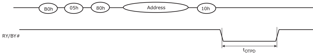
Figure 9.22 OTP Command (Page Protection Status) Timing Diagram
